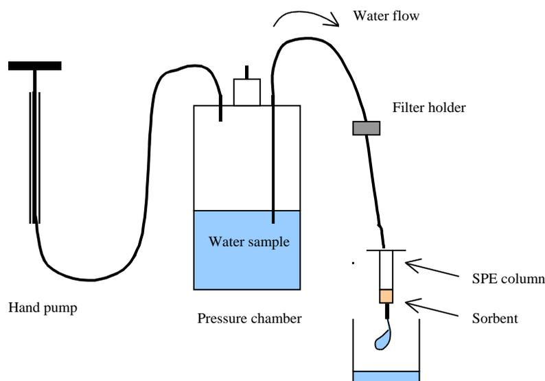
Figure 6. Pressure filtration apparatus used to extract pesticides from water in the field. Solid-Phase Extraction (SPE) columns contains a filter and a silica based sorbent having high affinity for non-polar compounds. In the filter holder a glass microfiber filter is placed to collect the particles in the water samples.
